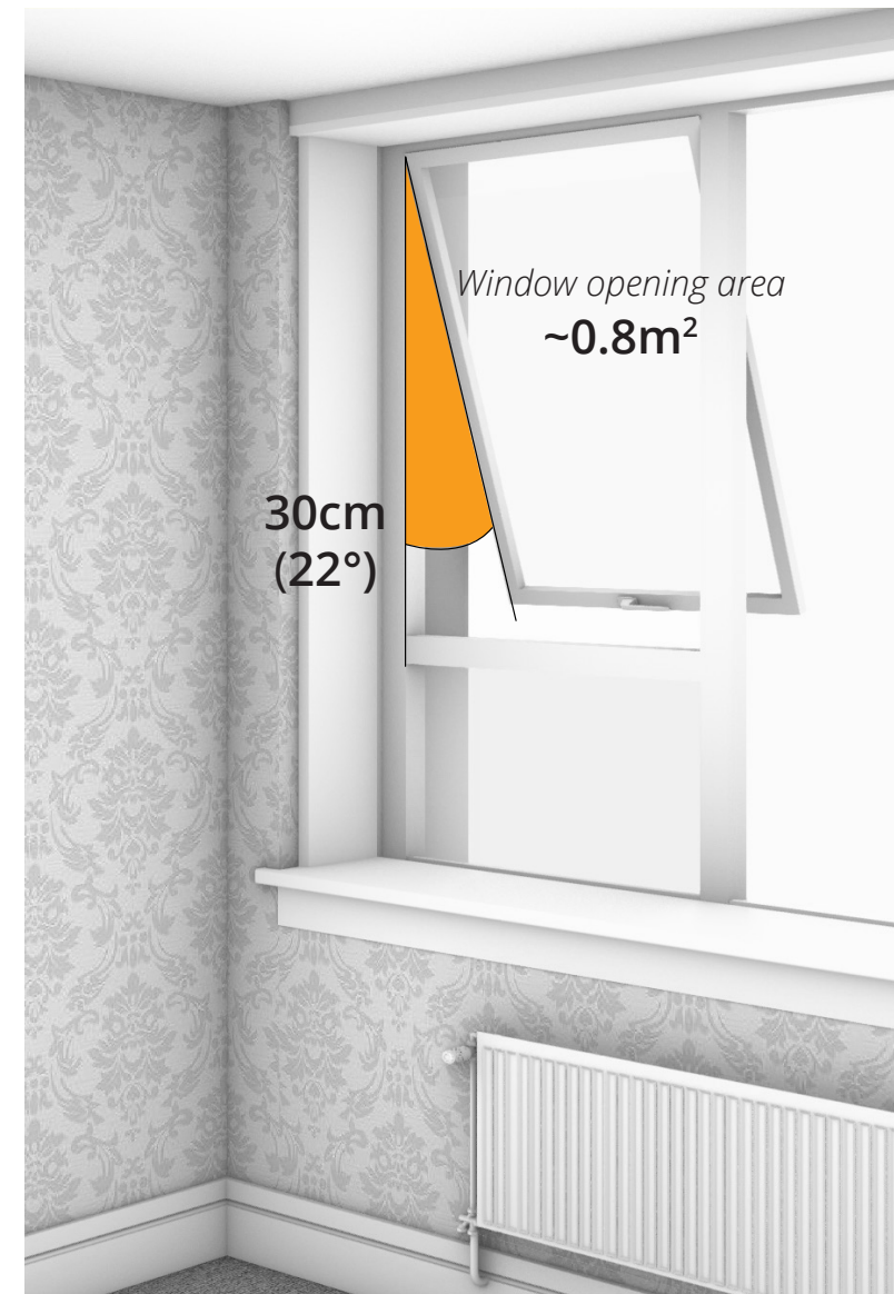
Existing windows Opening setting: 30cm
