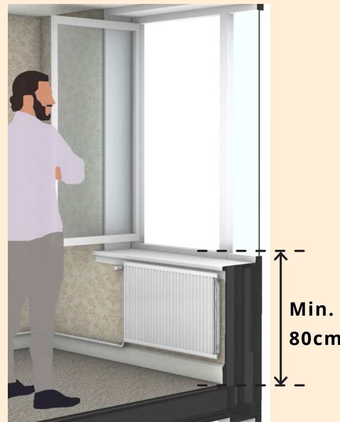
Regulatory guarding height below an open window
