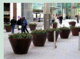
Planters can be used instead of bollards
