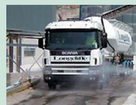
Wheel washing to remove dust and mud
