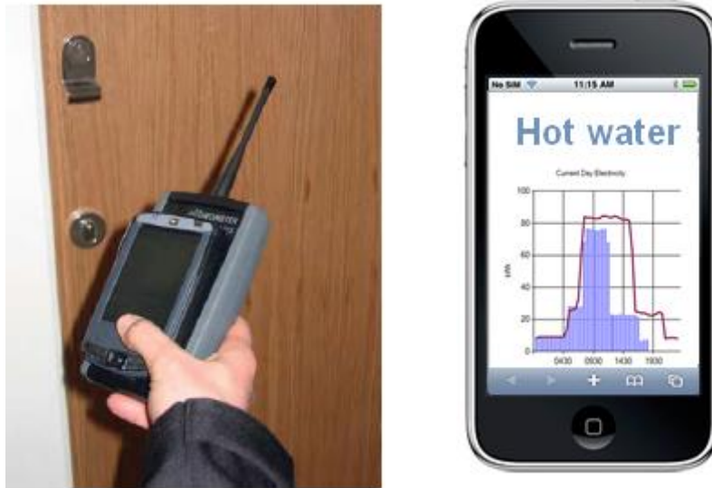
Figure 4: Wireless or automated meter reading can significantly enhance a district heating system in terms of efficiency and customer satisfaction
